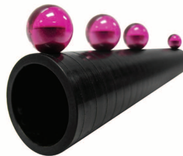
Calibrated ball arrangement to measure the sphere centre error
