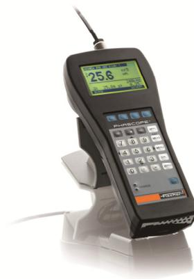
Fig. 3: The portable Phascope PMP10 uses the phase-sensitive eddy current measurement principle to determine accurately the thickness of TSA coatings.
