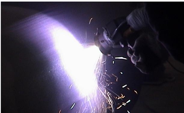
Fig. 1: TSA (thermally sprayed aluminium) coating process
