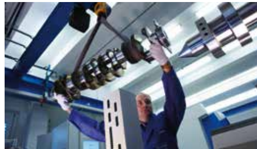
Use in production, loading a crank shaft with operator self-inspection
