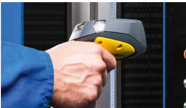
Barcode scanner for test plan selection and data input
