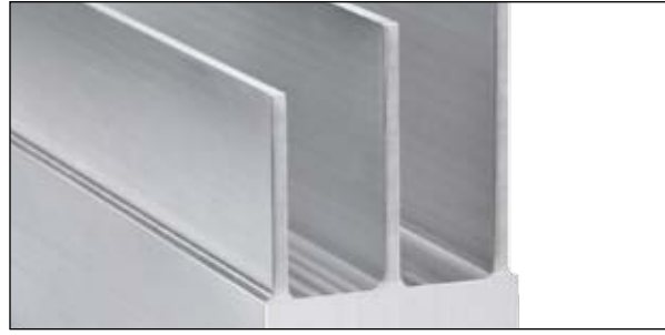
Abb. 5: Test workpiece made from aerospace aluminium 7075 l_3/d_1 ratio up to 5d_1 Step formation between two machining levels <0.006 mm Surface quality R_a <0.25 \mu\text{m}
