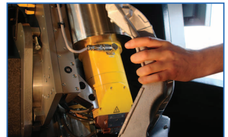
The unique 300 kV microfocus X-ray tube allows 3D scans even of large or high absorbing work pieces.
