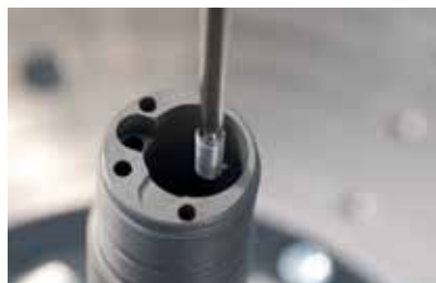
Form measurement in deep, narrow bores
