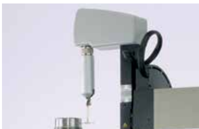
MDS4 with double-tipped probing system
