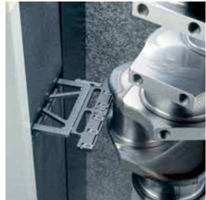
Flat measuring follower for crankshafts
