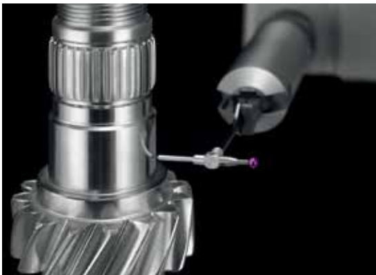
Twist measurement with a roughness stylus tip
