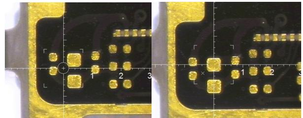
Fig.2: The programmed XY position is approached (left image); however, it does not exactly match the desired measurement target. The pattern recognition now looks for the defined image area and locates the correct measurement position (right).
