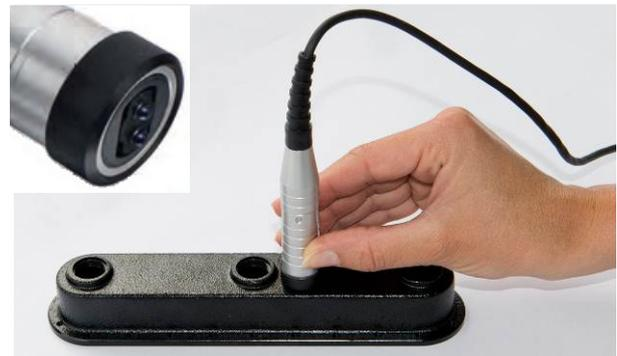
Fig. 2: Measuring lacquer on a rough surface with the V7FKB4 probe
