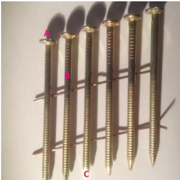
Fig.1: Zinc plated nails show measurement areas A, B and C. (Courtesy of Poppers-Senco Ltd)
