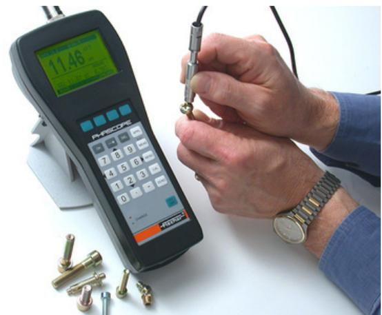
Fig.2: Measuring coatings on fasteners with PHASCOPE® PMP10
