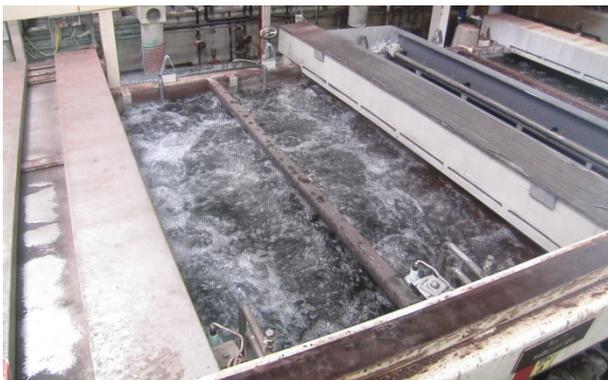
Fig.1: Analysis of a typical electroplating bath is especially important to guarantee a homogeneous coating process
