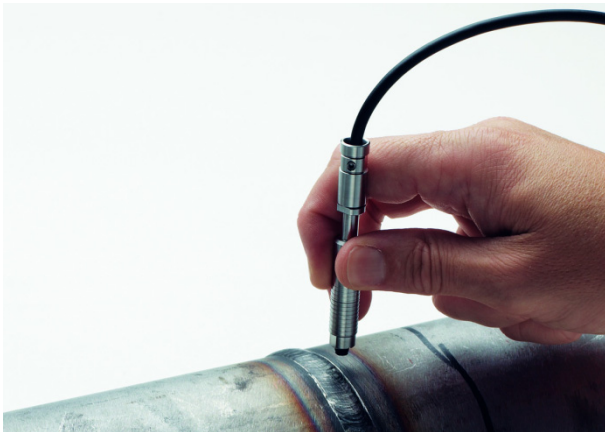
Fig.1: Measuring the ferrite content of a weld seam with FERITSCOPE® FMP30 and the probe FGAB1.3-Fe
