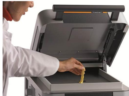
Fig. 2: Fast and non-destructive measurement of a gold wristband with the FISCHERSCOPE® X-RAY XAN® 220
