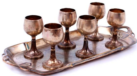
Fig 1: Tarnished silver, the tarnish may appear either uniform or spotty.
