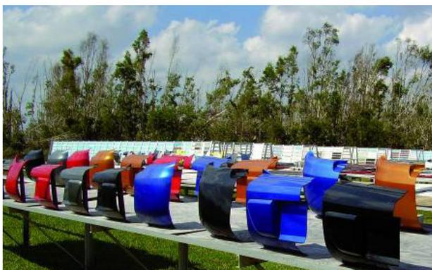
Fig. 1: Weathering rack in Florida of the company Atlas with various car body parts
