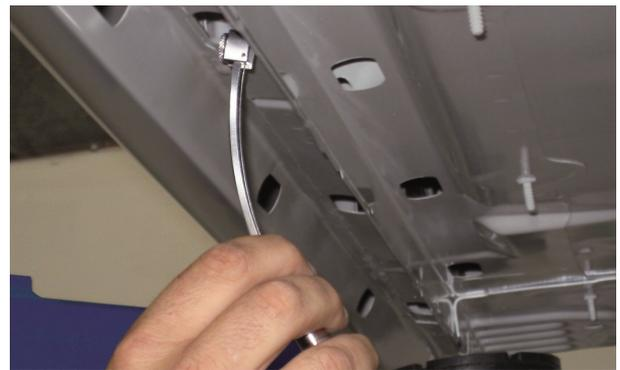
Figure 2: Insertion of the V3FGA06H probe into a hollow car body part to measure the CDP coating on the inside
