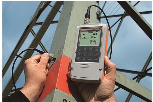
Fig. 2: Measurement of the duplex coating on electricity pylons using the DUALSCOPE® FMP100 and the FDX13H probe
