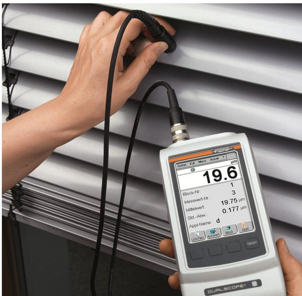
Fig. 1: Measurement of the coating thickness on blinds using the DUALSCOPE<sup>®</sup> FMP100 with the FTD3.3 probe
