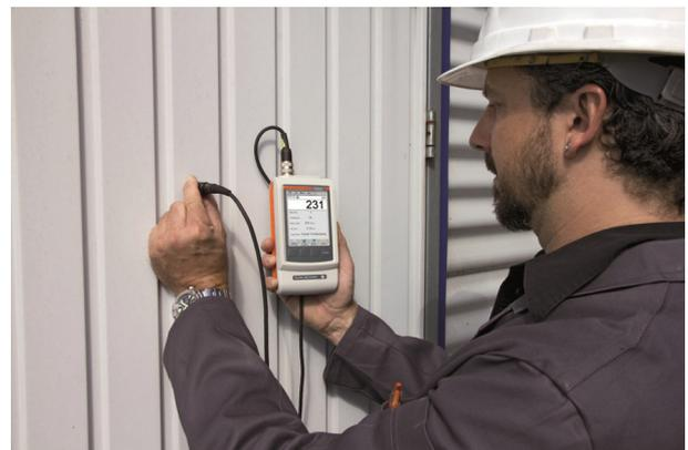
Fig. 2: Coating Thickness measurement with DUALSCOPE® FMP100
