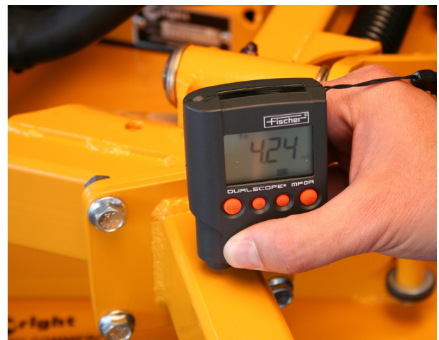
Fig. 1: The DUALSCOPE® MP0R is quick and easy to use yet extremely repeatable. Patented conductivity compensation allow for measurements on various non-ferrous alloys without time-consuming onsite calibration on the actual substrate material
