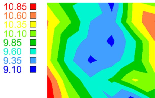
Fig. 2: Lateral coating thickness distribution of a specimen coated with only a few nm Au.
