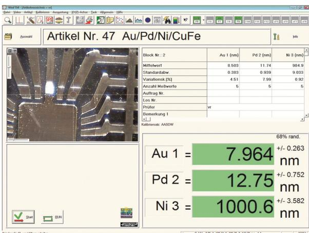
Fig. 1: High resolution measurement of an Au/Pd/Ni coating system on a leadframe and presentation of the results with the analysis software, WinFTM®.
