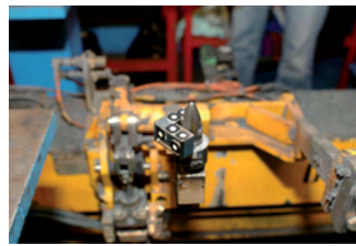
Fig. 6: TRITOP CM M cylinder adapter
