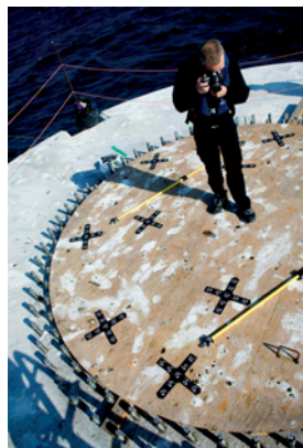
Fig. 12: Measurement with TRITOP CMM photogrammetric camera
