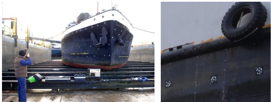
Fig. 2: The mobile optical TRITOP CMM system in use at a dry-dock. System and accessory can be easily transported by a single person. The system can be operated during measurement and evaluation without external power supply
