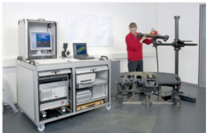
Fig. 3 ATOS 3D scanner designed for both metrology room and shop floor environments
