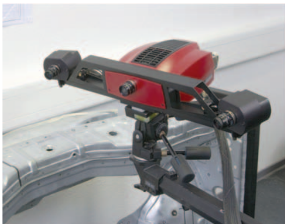
Fig. 3 ATOS 3D scanner designed for both metrology room and shop floor environments
